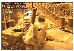
Two TOCDF workers place a mustard agent-filled 155mm reject projectile and its primary over pack container into a secondary over pack container to ensure the safe containment of the munition and its agent.
