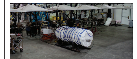
Ton containers (TC) await decontamination at PBTCDF at Pine Bluff Arsenal, Arkansas. Operators used magnetic induction heating to decontaminate 4,307 TCs, making them suitable for recycling.
