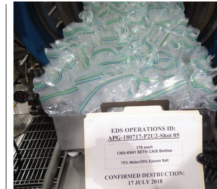
RCMD developed the CAIS bottle holder for the EDS, which can destroy up to 188 bottles in a single operation.
