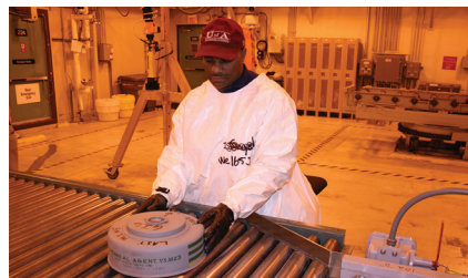
A munitions handler guides the last M23 VX landmine in the Anniston Army Depot stockpile as it heads down the conveyor.
