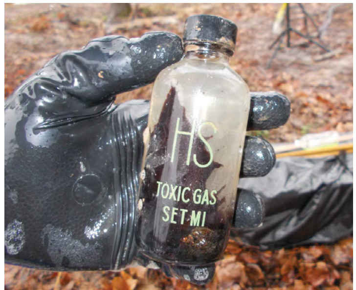
The U.S. Army has been directed to destroy CAIS, many of which were buried – an acceptable disposal practice until the 1970s. Pictured, a K-941 bottle containing concentrated mustard.
