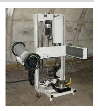
The Digital Radiography and Computed Tomography System uses X-ray technology to vertically scan a munition on a rotating platform to produce a digital view of the interior.
