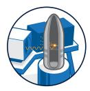
**Step 2**Neutrons penetrate container walls and interact with atomic nuclei, which emit radiation called gamma rays.
