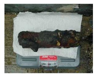
The 75mm projectile measures approximately 11 inches in length, three inches in diameter and weighs up to 12.5 pounds, depending on the type of chemical agent it contains. It also includes an adapter and booster casing that screw into the nose of the shell.
