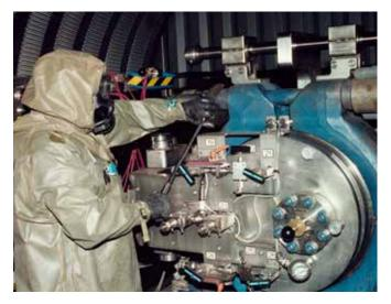
The EDS, seen here during the first DAFB mission in 2004, uses cutting charges to explosively access the chemical agent inside a munition and eliminate its explosive components.
