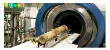
GTRs found to contain chemical agent are treated in the Pine Bluff Explosive Destruction System, which contains any blast, vapor and fragments within its stainless-steel vessel.
