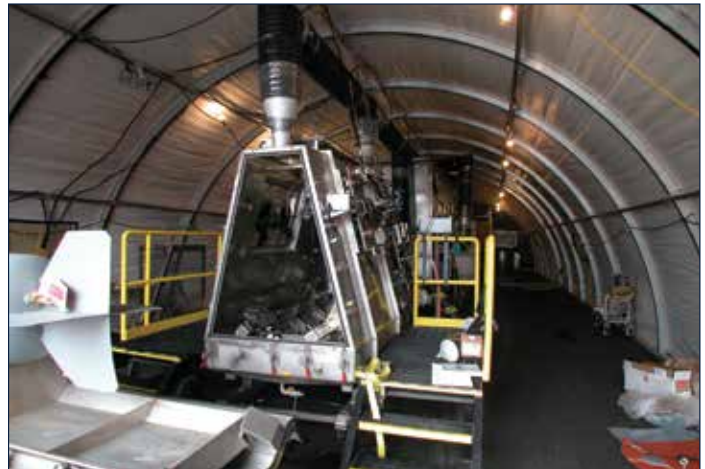
Located within an environmental enclosure, LITANS treats large RCWM items, such as 500-pound and 1,000-pound bombs and ton containers filled with chemical agent.
