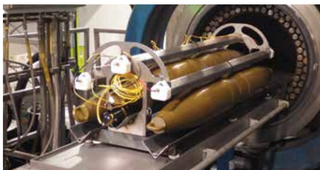
RCMD field testing of the EDS Universal Munition Holder, which can be configured to accommodate a variety of munition sizes and shapes.
