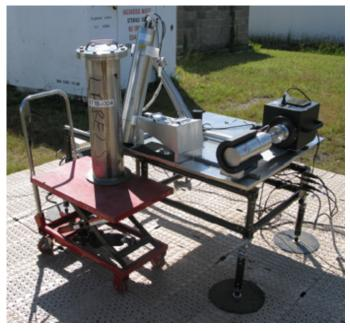
A recovered munition in an overpack container is positioned close to the NITIDS neutron generator. The neutrons penetrate the munition and interact with its contents, causing the atomic nuclei of the contents to emit gamma rays, which are detected by the system. Each element has a unique gamma ray signature that is used to identify the chemical fill.
