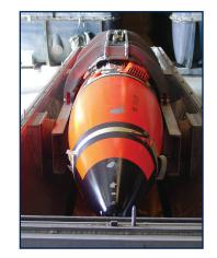
The TMU-28/B liquid agent spray tank is not a weapon, because it does not explode; rather, it is designed to disperse liquid nerve agent VX from underneath an aircraft. The tank's four major components are the agent container, aircraft suspension system, tail cone section and agent-dispersal nozzle. Spray tanks were designed to force air through nozzles to disperse agent as a fine mist.
