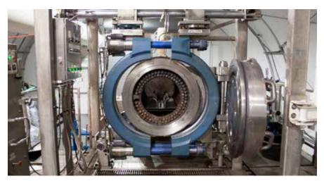
The Explosive Destruction System destroys recovered chemical warfare material while protecting workers and the environment.
