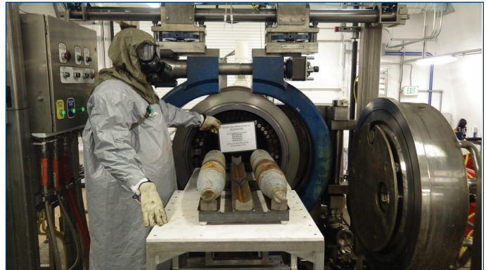
An operator holds an identification placard above chemical munitions set to be destroyed in the Explosive Destruction System, or EDS, in Pueblo.
