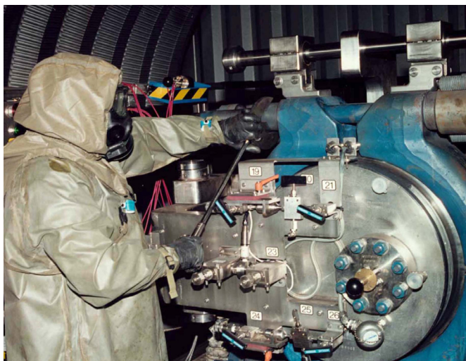
The EDS, seen here during the first DAFB mission in 2004, uses cutting charges to explosively access the chemical agent inside a munition and eliminate its explosive components before neutralizing the chemical agent.
