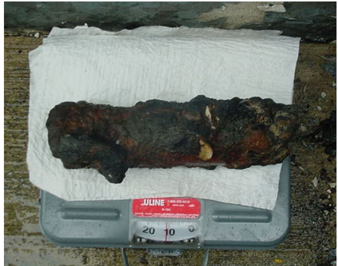
A 75mm projectile is approximately 11 inches long, three inches in diameter and weighs up to 12.5 pounds, depending on its liquid fill. This barnacle-encrusted munition was recovered at sea during commercial fishing operations.
