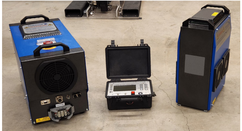
The high-energy X-ray generator consists of a power supply, an accelerator and a control panel.
