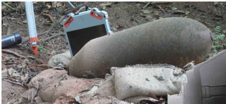
The high-energy X-ray generator allows for increased image resolution for thick-walled and overpacked munitions.
