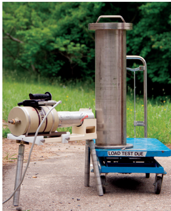
The Portable Isotopic Neutron Spectroscopy System quickly and reliably identifies compounds inside suspect chemical-filled munitions.
