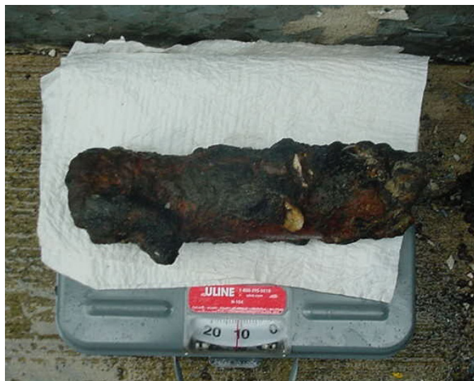
A 75mm projectile is approximately 11 inches long, three inches in diameter and weighs up to 12.5 pounds, depending on its liquid fill. This barnacle-encrusted munition was recovered at sea during commercial fishing operations.
