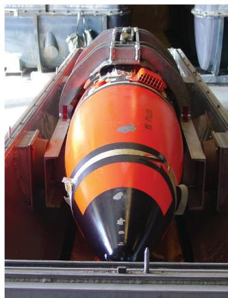
The TMU-28/B liquid agent spray tank is not a weapon, because it does not explode; rather, it is designed to disperse liquid nerve agent VX from underneath an aircraft. The tank's four major components are the agent container, aircraft suspension system, tail cone section and agent-dispersal nozzle. Spray tanks were designed to force air through nozzles to disperse agent as a fine mist.
